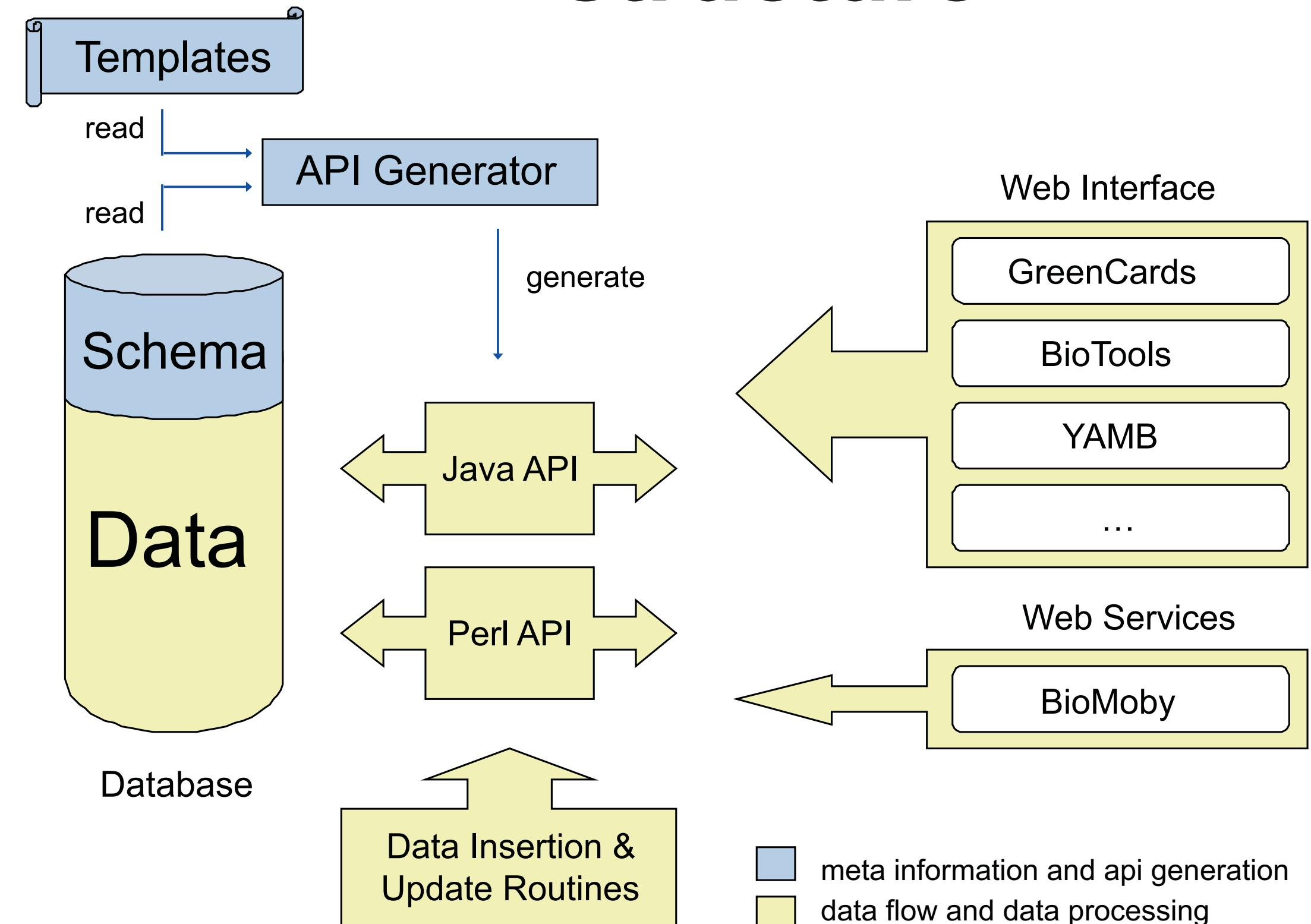
Schematic overview of the GabiPD application structure. The 'Templates' using the database meta-information (shown in blue), generating the database application interface (Java and Perl API). The application logic (shown in yellow), i.e., Web Interface, WebServices and data manipulation routines, interacts with the 'Database' through the database application interface.
